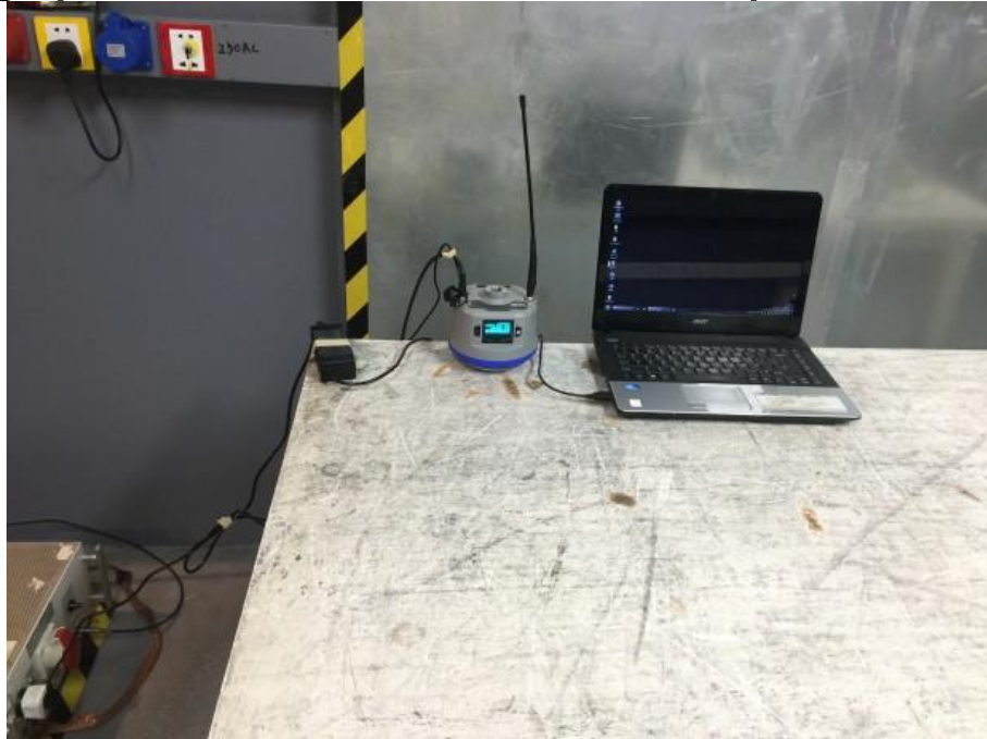
Photograph – Conducted Emission Test Setup
